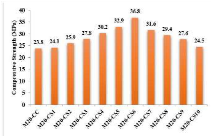
Fig. 3(a). Compressive strength of different copper slag M 20 concrete mixtures
