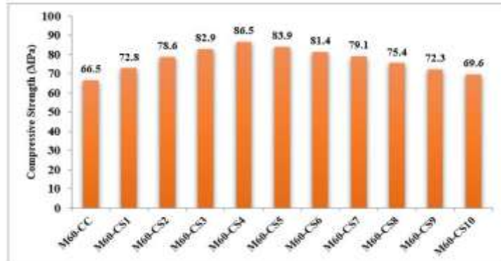
Fig. 3(c). Compressive strength of different copper slag M 60 concrete mixtures
